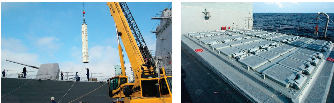
Figure 1. Missile canister being loaded into a vertical launch system (VLS), and a 64-cell MK41 VLS configuration aboard the guided missile cruiser USS San Jacinto (CG56), which has a total of 122 missile cells aboard. This canister weighs about three metric tons. The missile it contains is mechanically fragile and contains fuel and high explosives, so it is not loaded or unloaded at sea and not without good cause. VLS exists in a number of variations, ranging from just four cells to as many as the 64 shown here. San Jacinto has 128 missile cells, 122 of which can contain missiles and six that have strikedown cranes used for missile inspection and maintenance. (U.S. Navy images and Jane's (2020) , Naval Postgraduate School (2020) ).
